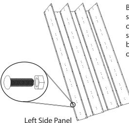
Bolt the tamper-proof screw on the inside of the locker. Only the screw heads should be visible from the outside of the locker.
