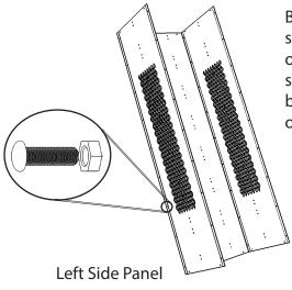
Bolt the tamper-proof screw on the inside of the locker. Only the screw heads should be visible from the outside of the locker.
